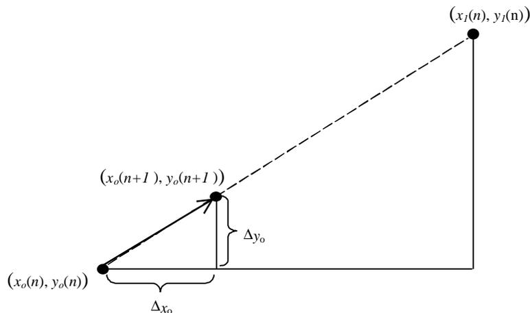
Figure 3: Movement by the chaser during the discrete time interval  $n$  to  $n + 1$ .
