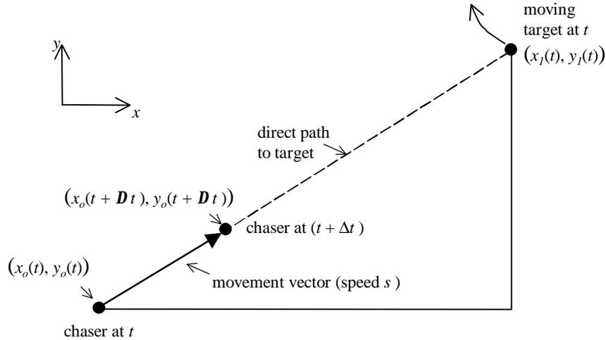
Figure 2: Movement by the chaser during the time interval  $t$  to  $t + \Delta t$ .
