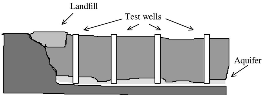
Figure 3: Bore holes for contaminant measuring equipment.
