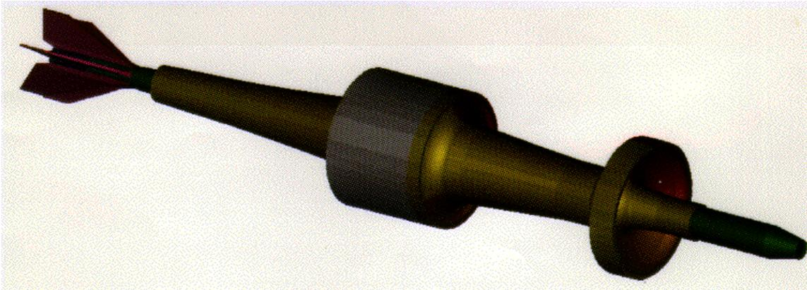
Figure 2. Computer model of penetrator with sabot, courtesy of ARL.
