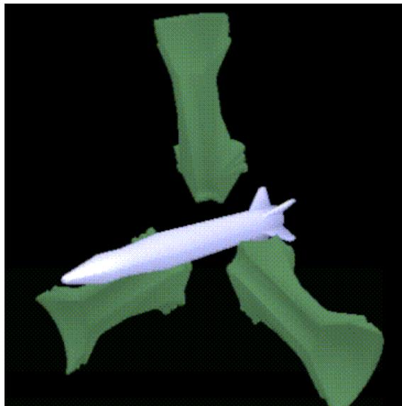
Figure 3. Model of sabot petal separation, courtesy of ARL
