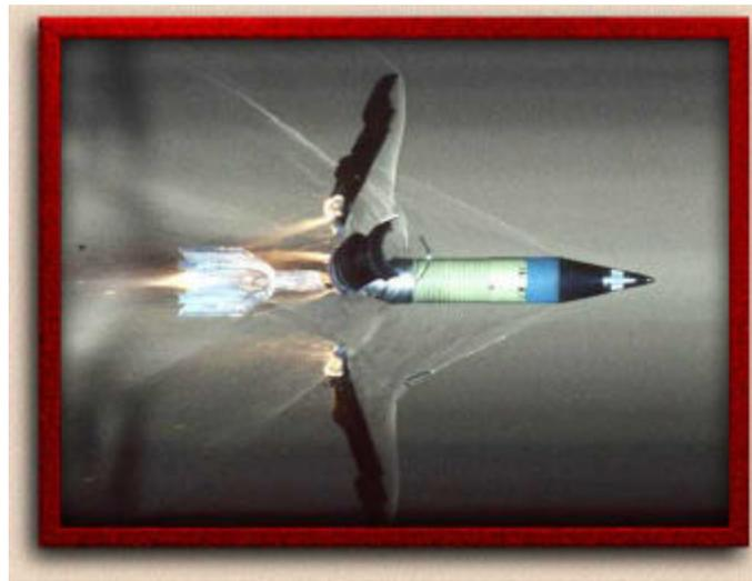
Figure 1. Tank round travelling in excess of 1500 meters per second, photo courtesy of Army Research Laboratories (ARL)
